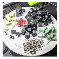
Here are listed all the TUTTO&SEMPRE components; most of them are already pre-soldered on the surface of the board (SMD). We just need to solder the through hole ones (THT).
