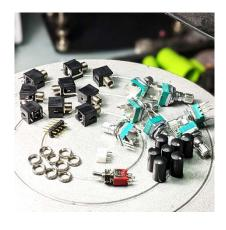
Here are listed all the SINGOLI components; most of them are already pre-soldered on the surface of the board (SMD). We just need to solder the through hole ones (THT).
