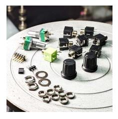
Here are listed all the ASCOLTA components; most of them are already pre-soldered on the surface of the board (SMD). We just need to solder the through hole ones (THT).
