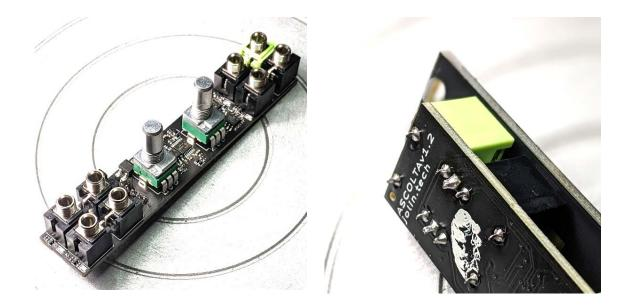
Position the **jumper** - the squared black piece of plastic - on the three pins header. Refer to the *manual* to choose where depending on your normalization needs.
