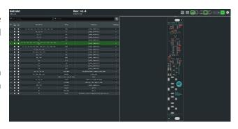
Here are listed all the GETREKT components, most of them are already pre-soldered on the board. We just need to solder the through hole ones (THT).
